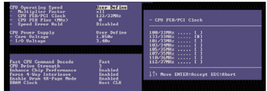
Figure 2-33 CMOS settings for front side bus speed
